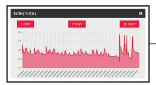
We monitor and store the voltage of the battery which is being used to power the Moving Intelligence (Phantom) tracking unit for 30 days, this enables you to spot possible issues with power drains, solar panel effectiveness and predict when your battery may need to be recharged.
